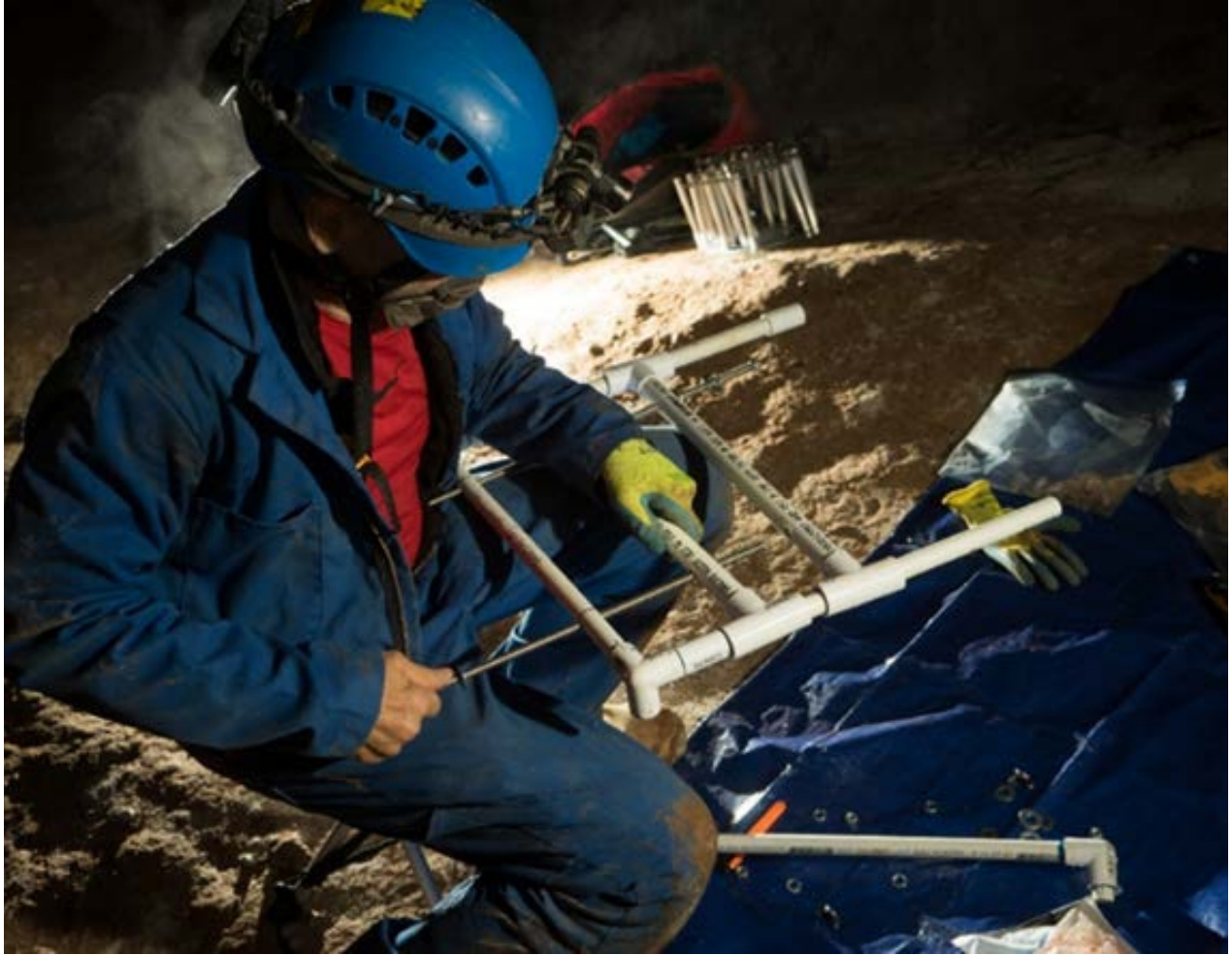
Mike assembling the Speleoclamp to hold the formation pieces while they are being drilled. Photo by Todd Roberts.
